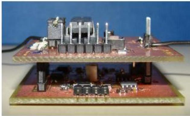
Fig. 6: Prototype implementation of the readout electronics required for TSM resonator sensors: the two units (microcontroller unit and analog front-end) are combined in a stacked setup.
