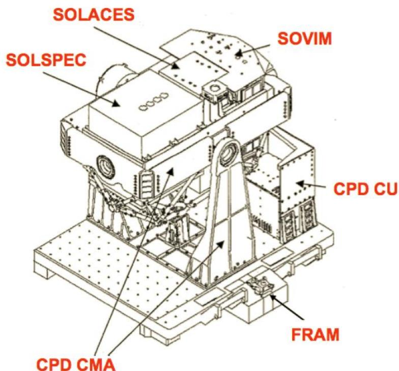
Figure1: the SOLAR package as it flies on the ISS COLUMBUS module, the supporting platform (FRAM and CPD) aims solar pointing during the solar visibility periods.,
